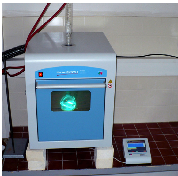
Fig. 2. The microwave photocatalysis arrangement on Milestone's MicroSYNTH Lab-station.
